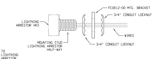
STEP 7. INSTALL LIGHTNING ARRESTOR ASSEMBLY AS SHOWN BELOW;
