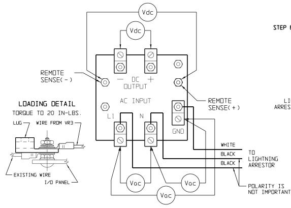
NOTICE. TO INSTALL OR REPLACE THE LIGHTNING ARRESTOR OPTION ON THE ATIO SERIES BATTERY CHARGER IS NECESSARY TO FULLY REMOVE THE SHROUD AND THE INSTRUMENT PANEL. PROCEED WITH THE FOLLOWING INSTRUCTIONS.
