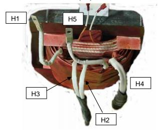
It shows the transformer (T1) connection set up for 240Vac input. The wires from the ac input circuit breaker (CB1) will be going to H1 and H5.
