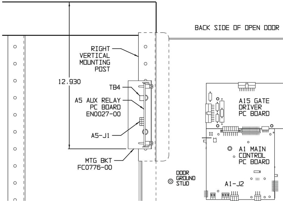
**Figure 1 - front view of properly installed components**
