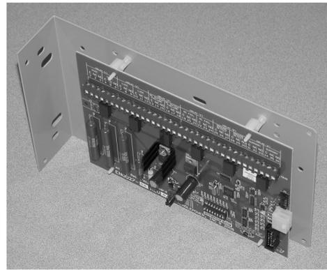
**Figure 3 - A5 pc board mounted on bracket**
