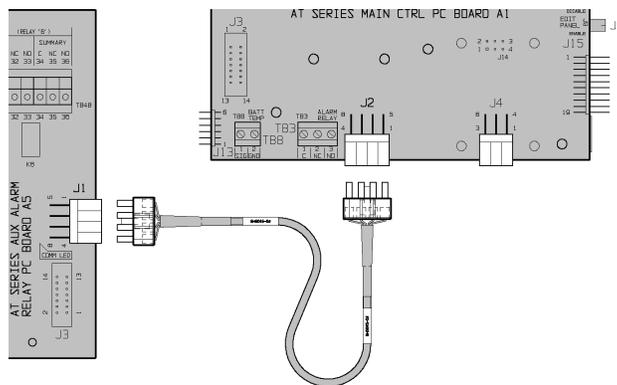
**Figure 4 - serial cable interconnection**
