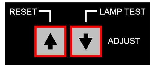
The reset function will clear all latched alarms and de-activate the Summary Alarm relay contacts (TB3). If any alarm is *still active* while performing the latch reset, that alarm's associated LED indicator will *remain* lit after the latch **RESET** button is pressed. The alarm will latch again after 30 seconds, and the Summary Alarm relay contacts will switch to the active state.
