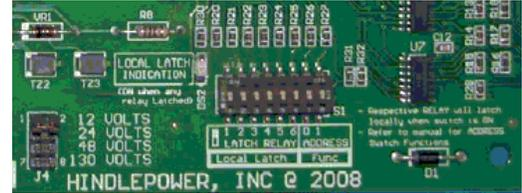
The first six (6) switches (1-6), labeled **Local Latch**, correspond to the individual auxiliary alarm relays physically installed on the pc board (A5). These relays are labeled along terminal block (TB4), with individual alarm relay contacts marked in the non-alarm condition. They are as follows:
