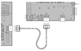
Figure 4 - serial cable interconnection
