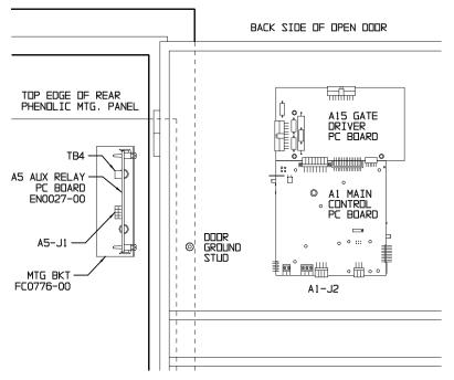
Figure 1 - front view of properly installed components
