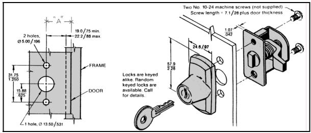
4. On Style-586 & Style-594 enclosures, the hole pattern (shown above) must be rotated 90° clockwise.
